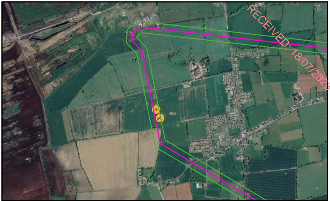
Figure 15.11: Existing overhead power line ( in pink ) relative to recorded monuments ( orange dots ) and associated Zones of Notification ( shaded yellow ) in Clonin townland near Rhode village, Offaly (50m radius to either side of power line shown in green ).
